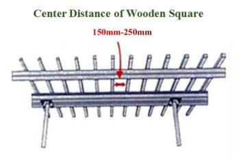
(1) Wood batten and vertical rib of Board should mutually perpendicular fixed.
